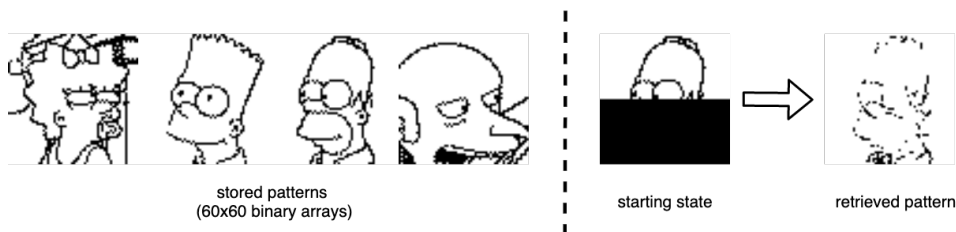
Figure 7: Pattern retrieval error in a Hopfield network.
